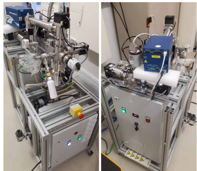
Figure 1: Mobile pumping units.
