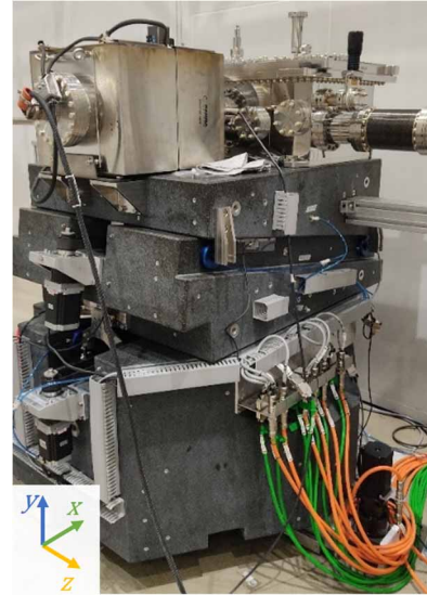
Figure 1: Mirror granite bench design used as a reference.
