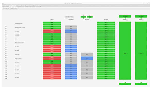
Figure 1: Inputs Beam Interlock System.
