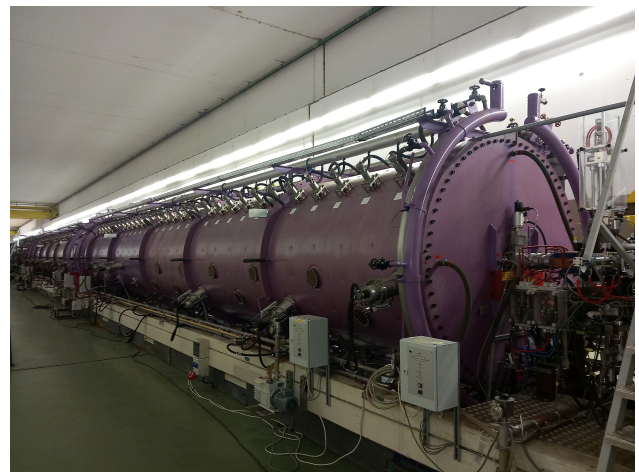
Figure 1: The Alvarez type main linear accelerator of the UNILAC went into operation in 1975.
