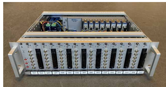
Figure 2: A photograph of a pilot subrack for the replacement of Bitbus based controllers using an NI-cRIO controller and custom-made DIF and IFA cards.
