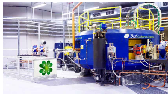
Figure 2: The 70 MeV cyclotron apparatus used as source for the proton line in the ISOL facility.
