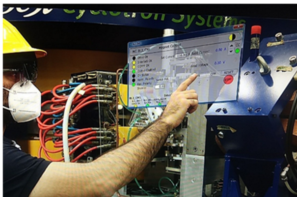
Figure 1: Human-Machine Interface through AR technology for cyclotron supervision.
