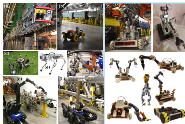
Figure 1: Overview of CERN's robots: (a) Train Inspection Monorail (CERN-made), (b) EXTRM robot (CERN-controlled), (c) CERNBot in different configurations (CERN-made), (d) drone for tele-op support, (e) quadrupeds for challenging terrain, (f) high-payload industrial arm for milling and repetitive tasks, (g) TEODOR robot, (h) Telemax robot.
