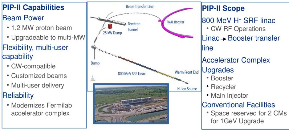
The PIP-II scope enables the accelerator complex to reach 1.2 MW p-beam on LBNF target
