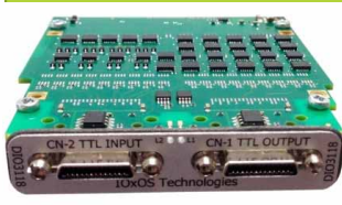
16 channel input and 16 channel output
