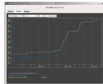
Working hours of a hoist over time
