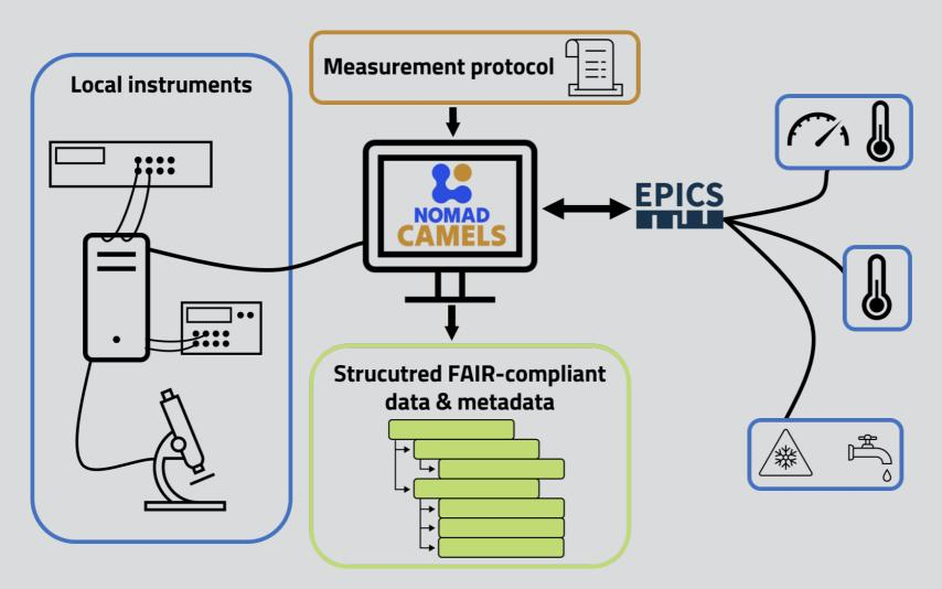
Fast communication with local measurement instruments allowing for real-time visualization of the recorded and time-stamped measurement data
