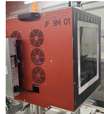
PSI JUNGFRAU 9 Mpixel @ 2 kHz 36 GB/s detector
