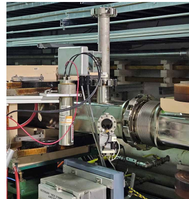
Thick secondary foil in the injection section of the proton accumulator ring
