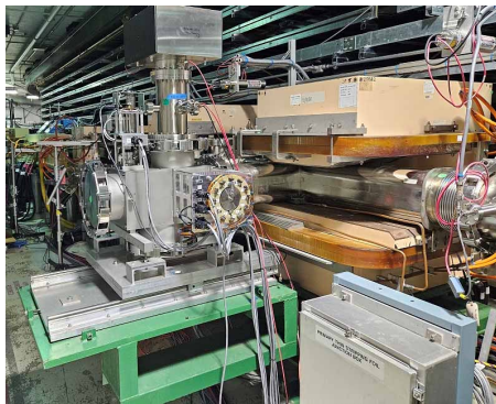
Thin stripping foil in the injection section of the proton accumulator ring
