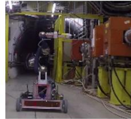
Remote radioprotection surveys
