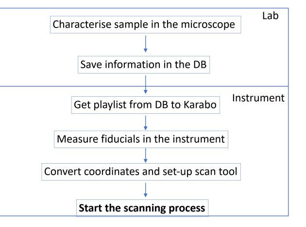
Karabo integration guides users through an automated workflow: V 🗙
