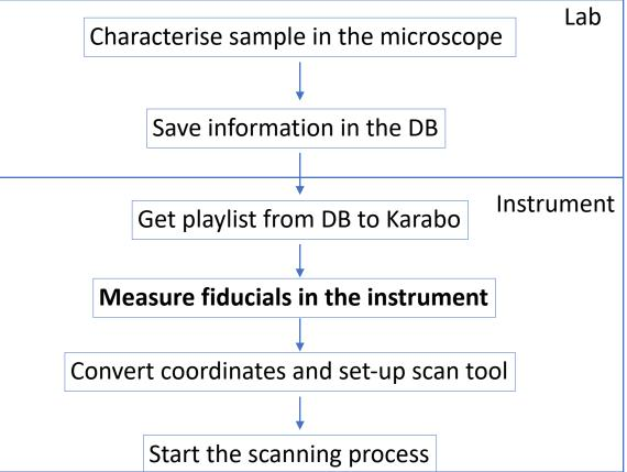
The target coordinates are located along with the fiducials in the laboratory prior to the experiment. Relational database stores target and fiducial coordinates for easy management. Information is directly accessible via the Karabo control system Fiducial measurements are performed in the instrument Target coordinates are transformed from the lab base system to the instrument base. The transformed coordinates are then sent to the Karabo scanning tool.
