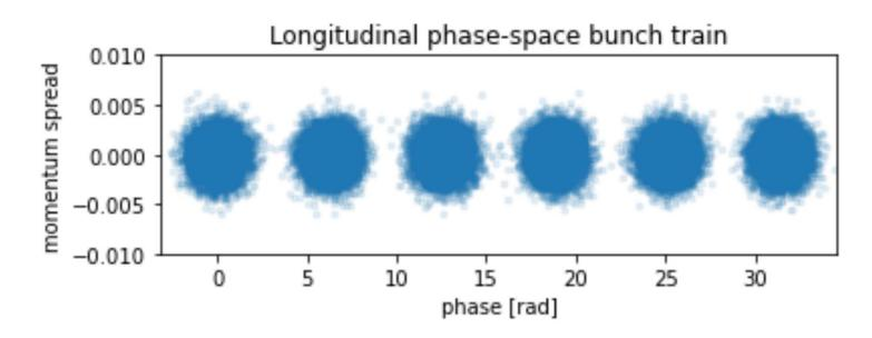
Example of six 80-nanosecond bunches constituting one full orbit (i.e.,  $12\pi$  rads in phase) at 400 kHz revolution frequency. Each bunch is a 2D Gaussian distribution of 10,000 particles (variable).
