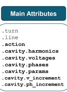
.cavity.voltages and .cavity.phases change during execution according to .cavity.v\_increment and .cavity.ph\_increment , respectively
