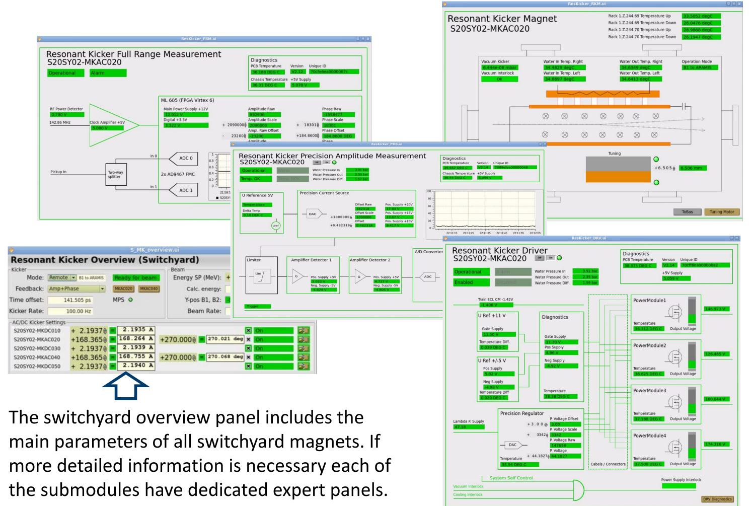
The goal of Synchronisation and Timing system is to synchronize the kicker with the electron beam, Driver provides the kicker excitation power, Full range measurement provides pulseto-pulse amplitude and phase information about the oscillating current, Precision measurement system provides higher resolution measurement the kicker's of current amplitude.
