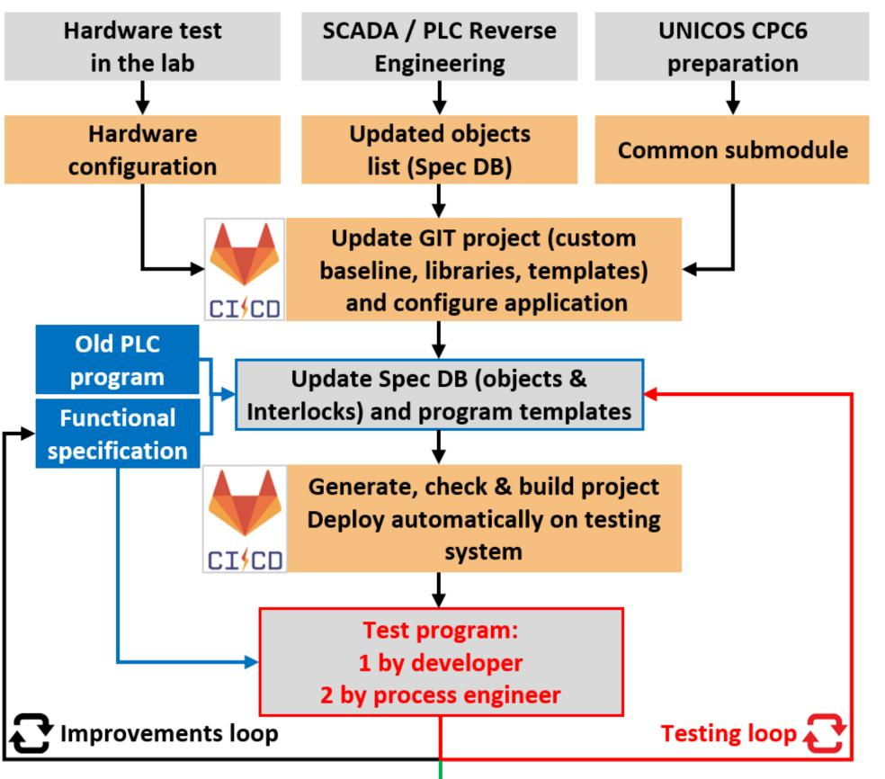
The development of the LAr control software was based on the unified software production process presented in **THPDP065**. Since the software production is fully automated, the main tasks of the developers, were to provide a tested PLC hardware configuration, complete the UCPC6 objects list, and program code templates. Each commit to the GitLab repository triggers CI pipelines that include project generation, checks, builds, and automatic deployment to the PLC-SCADA testing environment.
