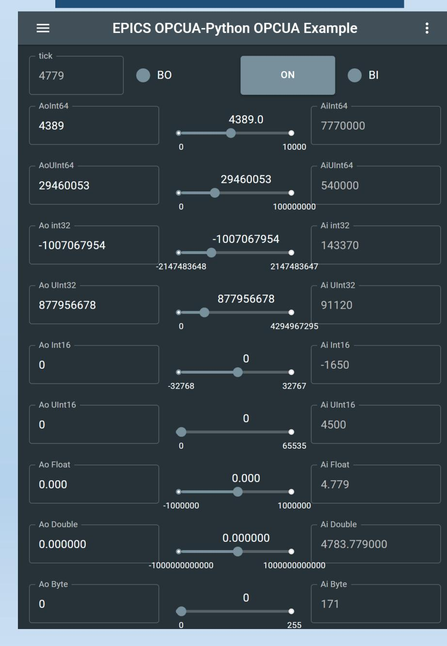
An OPC UA to EPICS bridge that has been containerized with Docker to provide a microservice for communicating between EPICS and OPC UA variables has been designed. The system supports all the standard OPC UA data types. We urge the EPICS community to test and evaluate the system and to provide feedback via the React-Automation-Studio discussion group[19].
