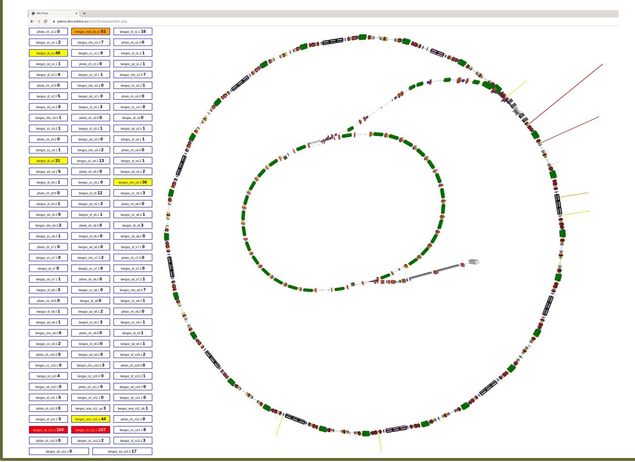
DODECAGON is an SVG based application in which each of the 12 sections can be selected. Users can switch ON, OFF and standby High Voltage power supply and/or Feedbacks and set a value using the knob component
