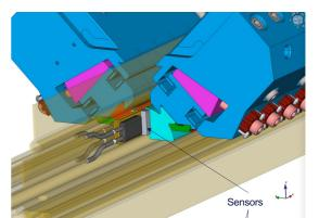
The two bilateral sensors are equipped with 0.5 mm thick steel tapes. These tapes are used for two purposes. First, the attractive force of magnets is to be used to position the sensor in the gap. The second is to create a gap of about 0.5 mm between the surface to be measured and the sensor.
