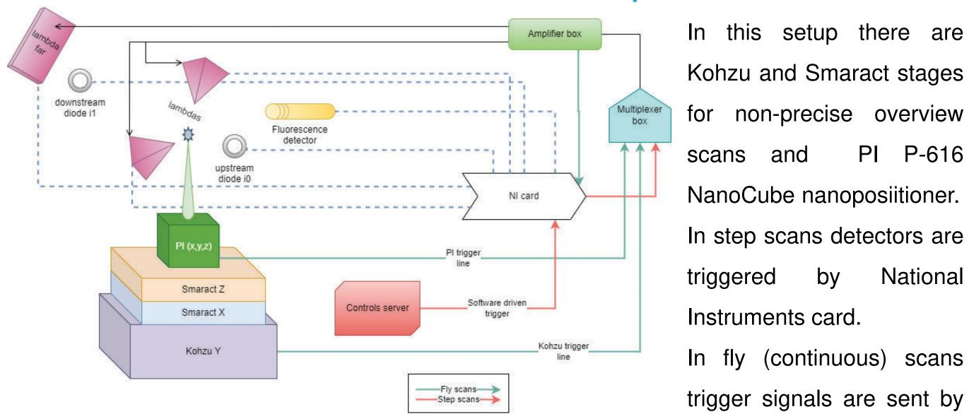
Kohzu and Smaract stages for non-precise overview PI P-616 scans and NanoCube nanoposiitioner. In step scans detectors are triggered National Instruments card.
