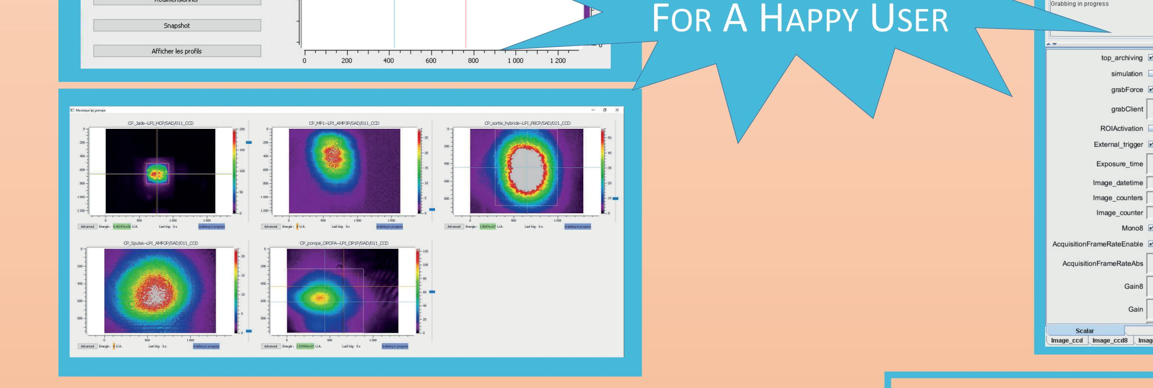
The DevCalculs device associated with DevPylon and DevVimba allows a real-time computation of centroid, alarm zone, local maximum, etc. and also displays userdefined references.
