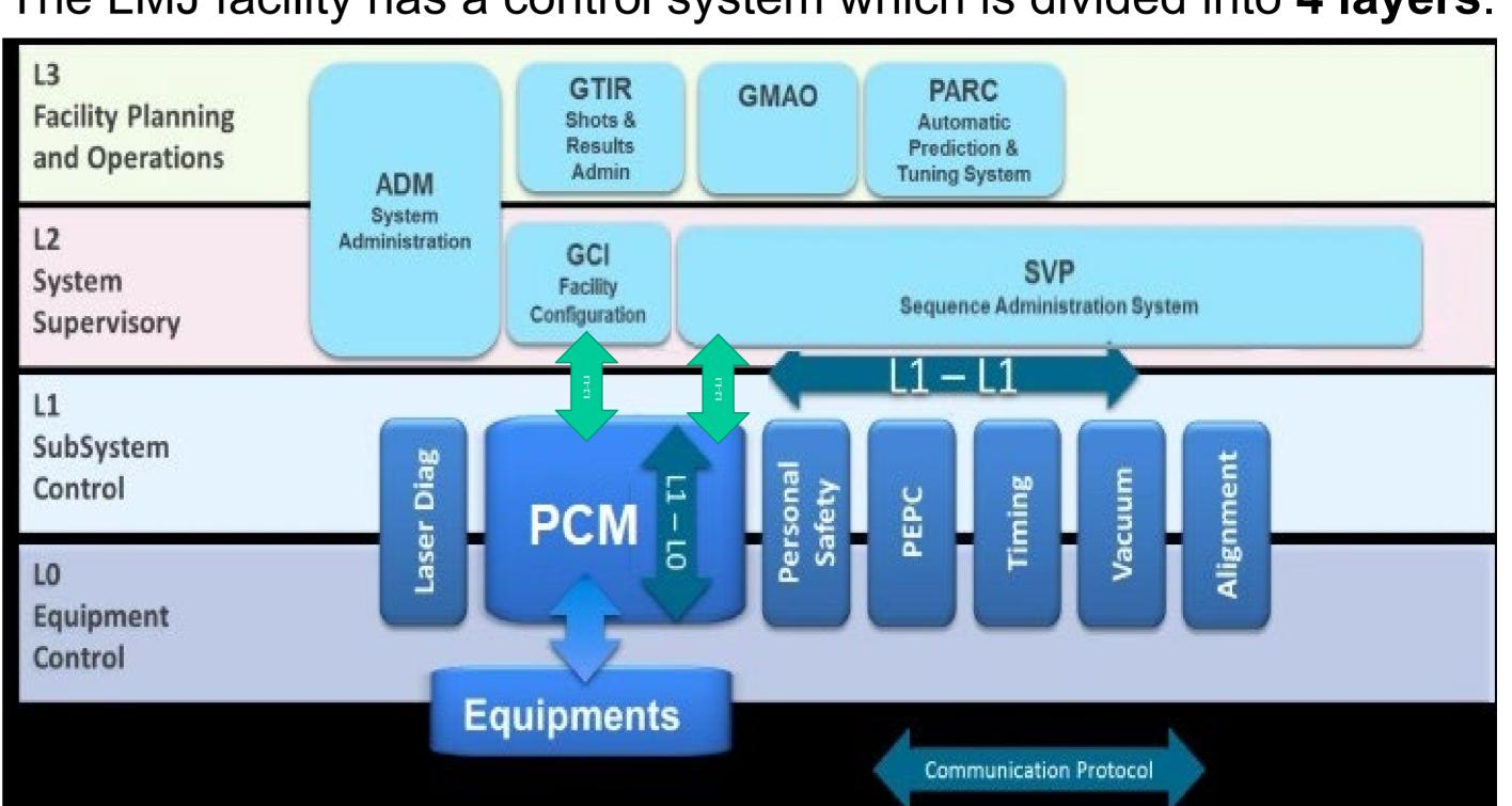
The <u>L1 and L0 layer</u> are divided into <u>12 major subsystems</u>, corresponding to the main functions of the LMJ beam's control system. The <u>PCM CS</u> receive shot parameters from facility Configuration software, called GCI and from sequence administration system, called SVP.
