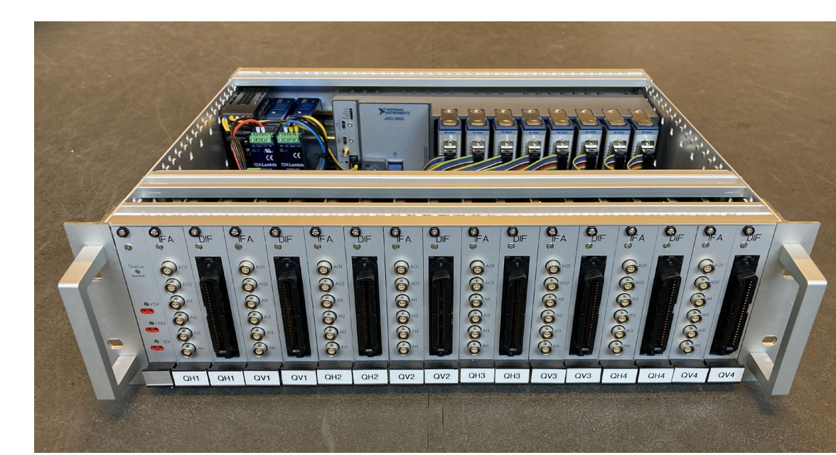
NI-cRIO subrack for controlling eight power supplies
