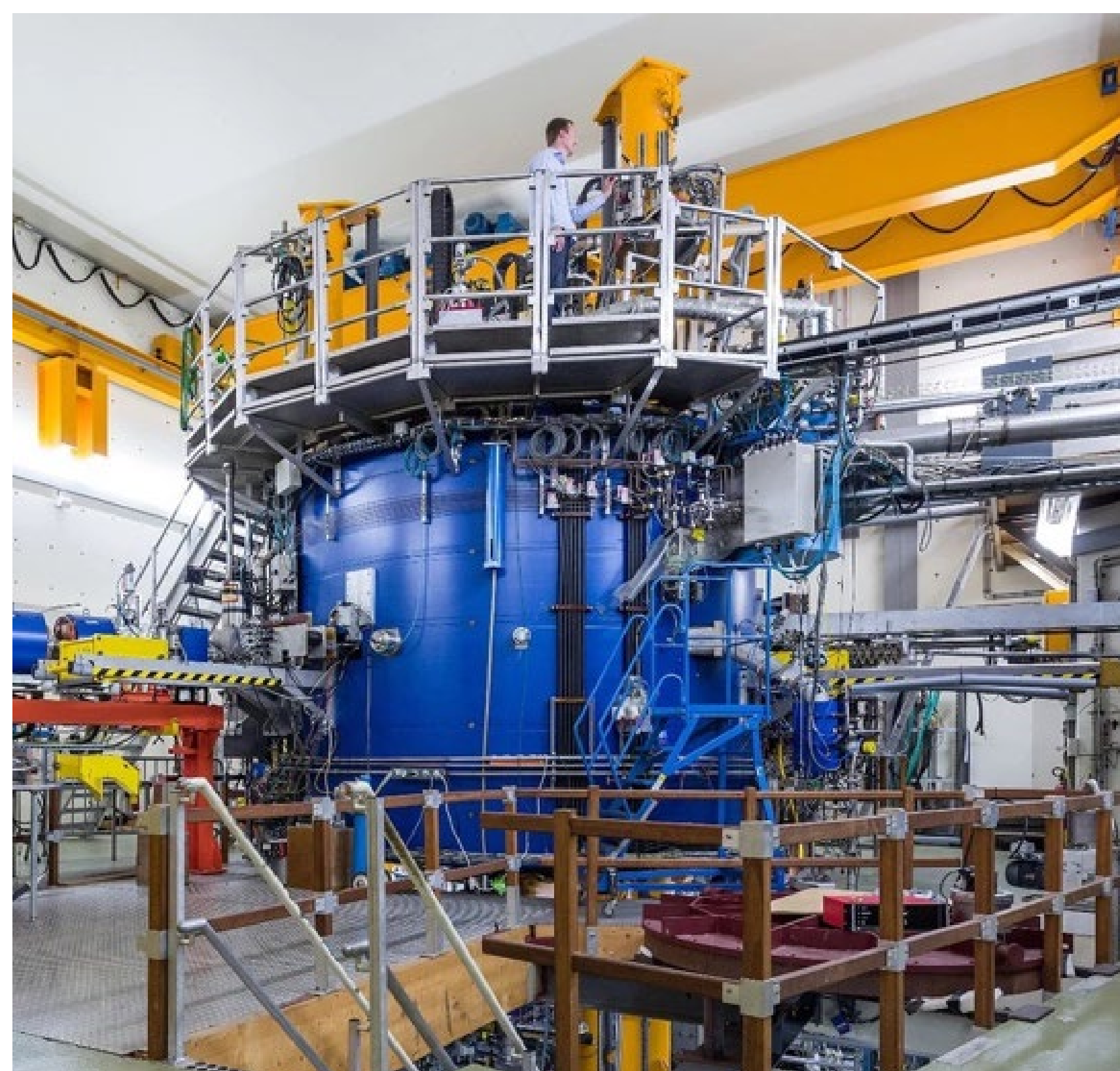
The AGOR superconducting cyclotron of PARTREC, delivering beams of high energy protons and other ions.
