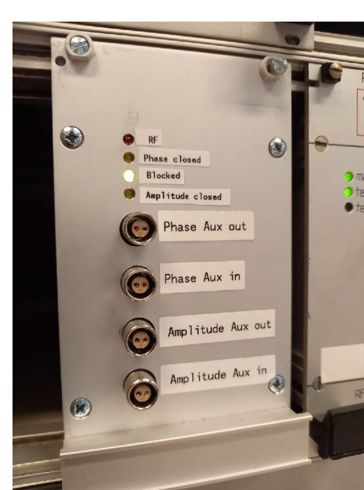
Redesigned module with all functions combined into one cassette
