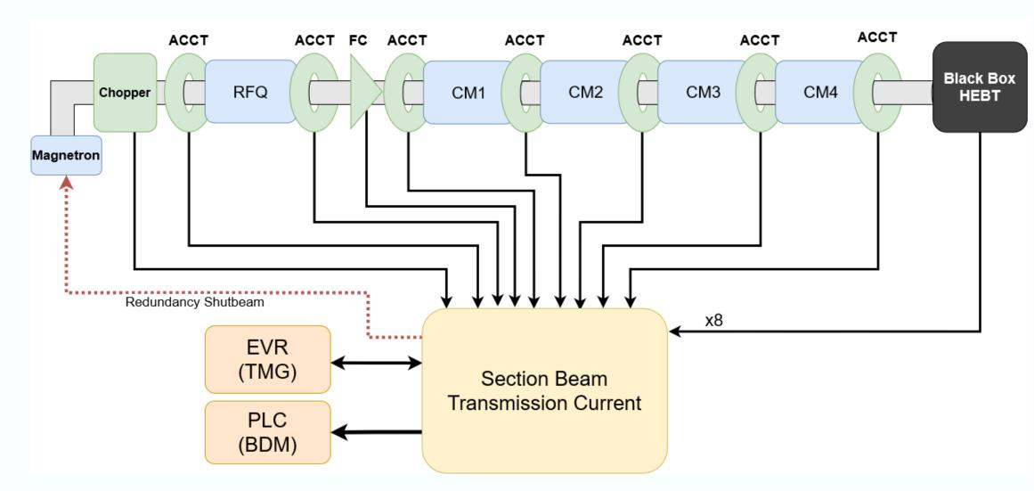
The SBCT acquires beam current in the accelerator from different ACCTs, and Faraday Cup, and also the chopper voltage
