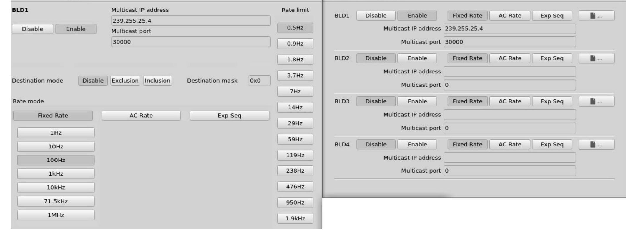
Up to four BLD rates can be configured simultaneously, each accessible at its configured IP destination and port, with a maximum rate of 1 MHz. Up to 31 32bit processed data variables can be sent upstream per event. If proper care is not taken when tuning BLD, the upstream network bandwidth may get saturated easily, as well as the CPU usage.
