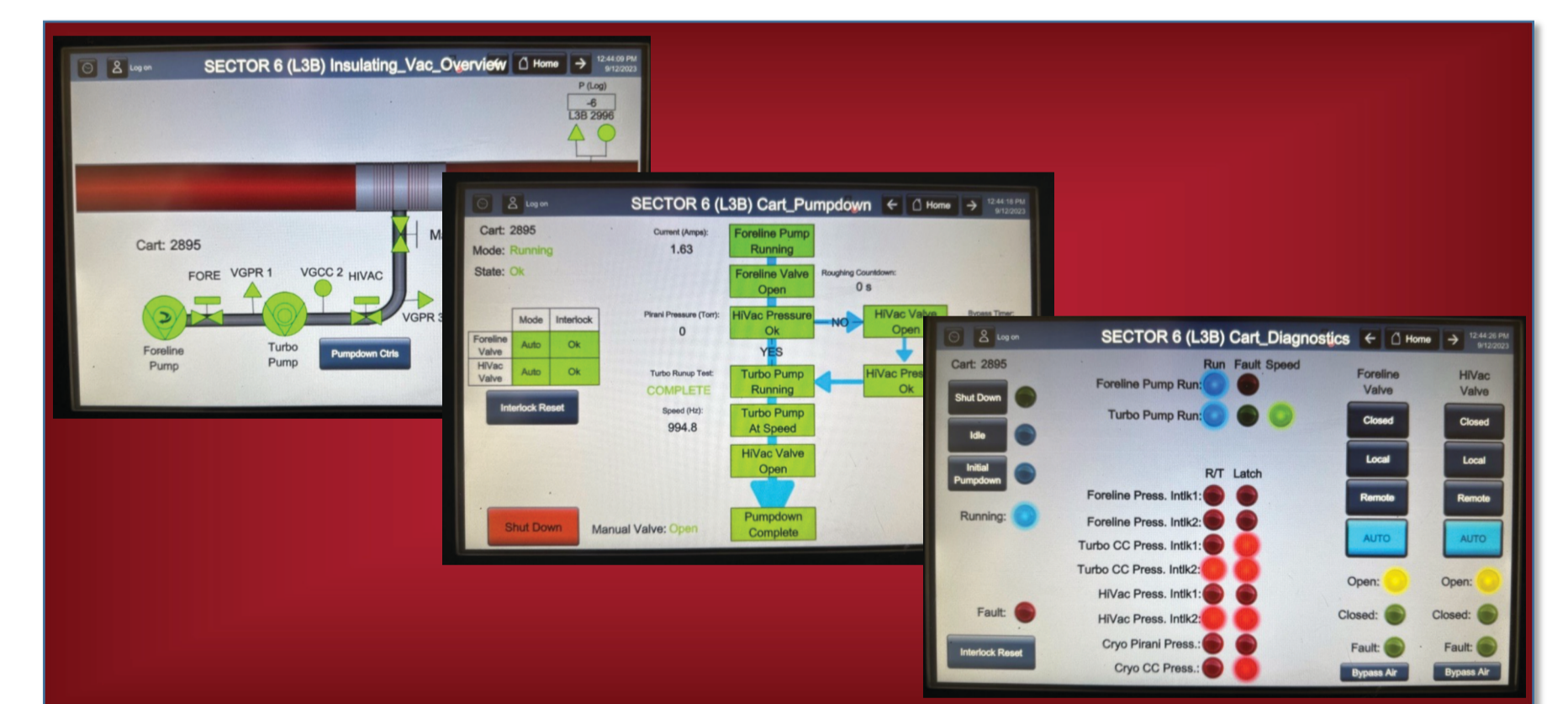
PLC touchscreen HMI screens.
