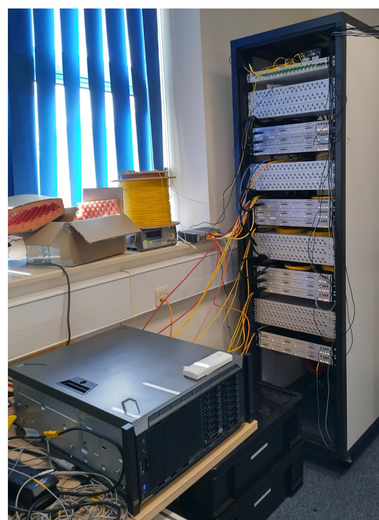
Full scale prototype. 10 digitisers + server + WR timing
