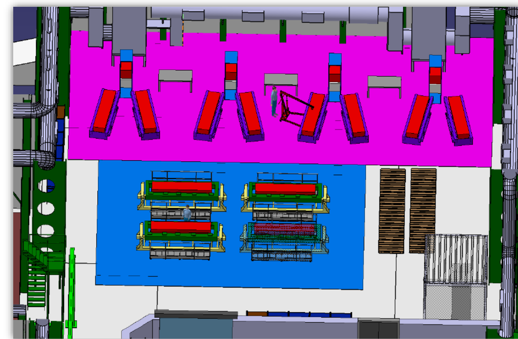
Fig. 9.: Drawing of the future Integration stand during the EB refurbishment, with the layout of 4 racks and 8 supermodules.
