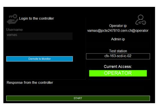
When correctly logged in, the software subscribes to the master launcher to obtain information of each module running on any of the controllers. If found, it tries to establish communication with all data channels as well as to the channel information. The master launcher also publishes the information about the host panels allowed to operate selected test bench, to block the possibility of operators controlling the hardware that is not connected to the specific test bench.
