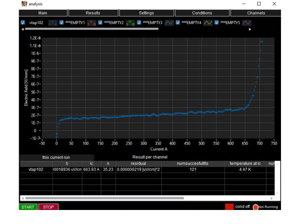
The microservice based software for characterizing superconductors has been successfully implemented, commissioned, and deployed at CERN. It can effectively evaluate both low-temperature superconductors such as NbTi and Nb3Sn, and high-temperature superconductors such as MgB2 or REBCO, both before and after the production of superconducting cables.
