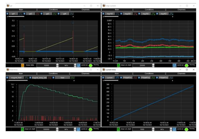
All the users can run monitoring modules such as time value plots, or time value saving modules, where the users identify signals to plot or to save. The operators can run modules to show sample power, magnet power, interlock security control or control channel to have a full control of the program during the test.
