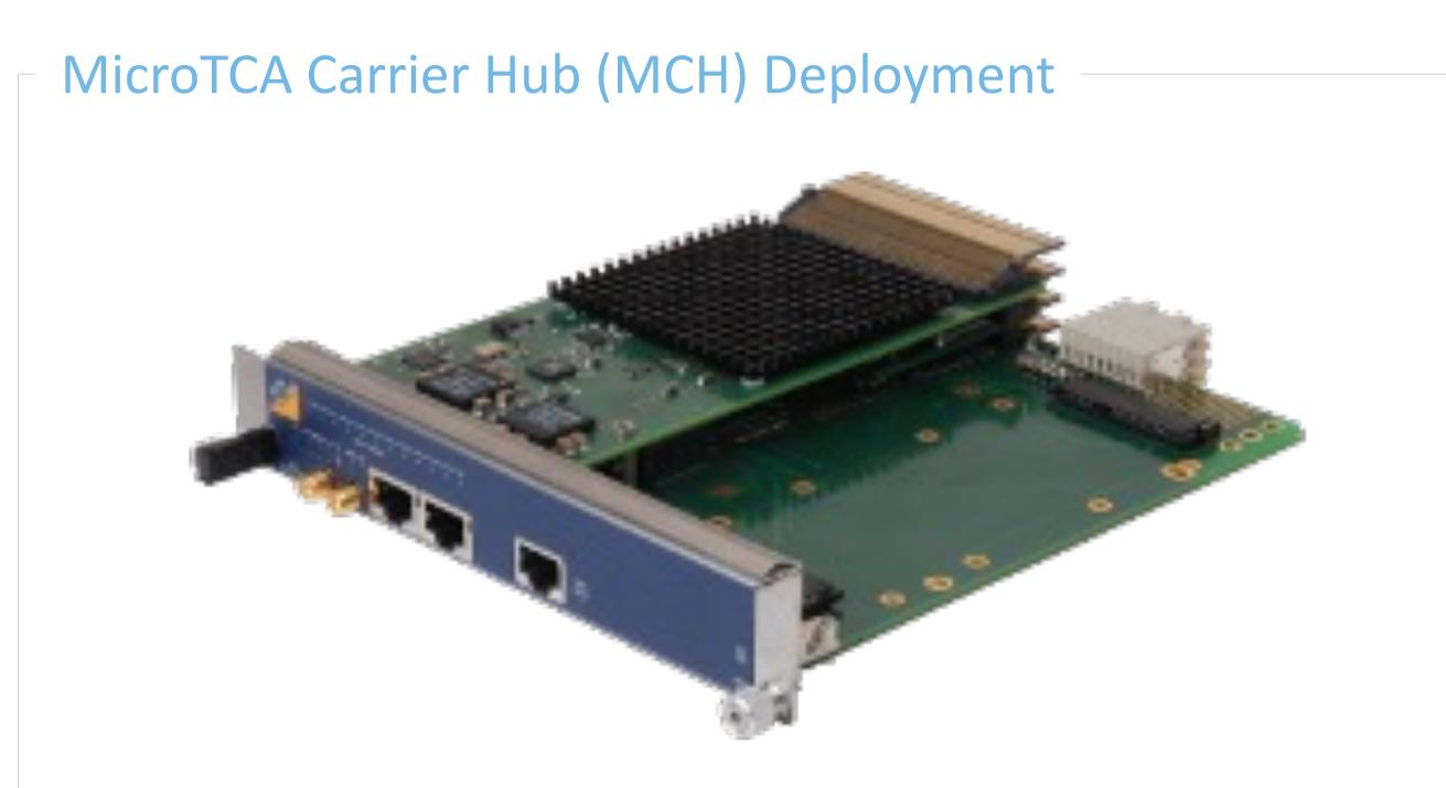
The MTCA Carrier Hub used at ESS is the NAT-MCH-PHYS board.
