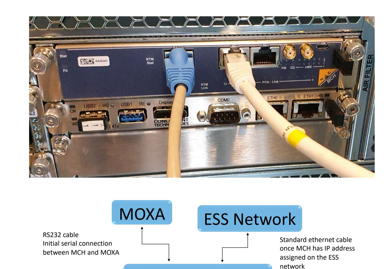
Initial configuration is done via RS232 through MOXA server, to allow a serial connection between the unconfigured MCH and the ESS network. Next step is the registration of the MCH on the ESS network, which is done in a custom in-house configuration management tool (CSEntry) REST API.
