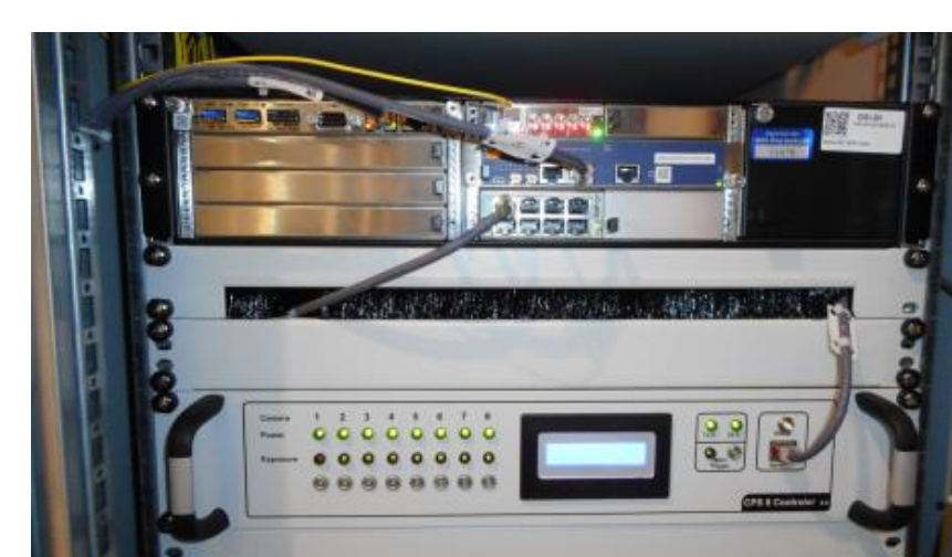
Figure 10: Scintillating screen DAQ system
