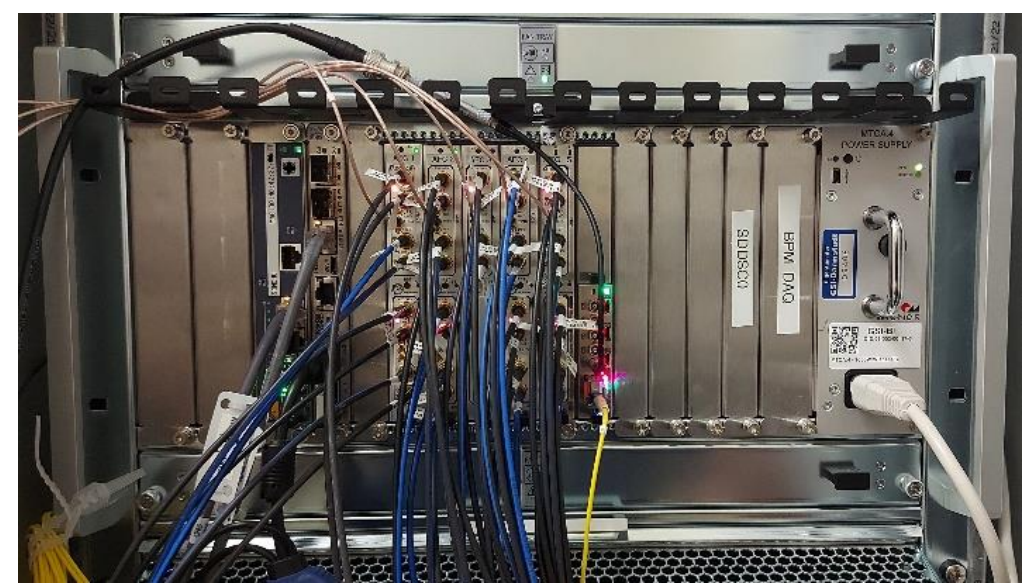
Figure 3: CRYRING@ESR Beam Position Monitoring system using AFC V3.1 FMC carrier modules with 250MSa/s/4Ch/16 Bit ADC FMCs.
