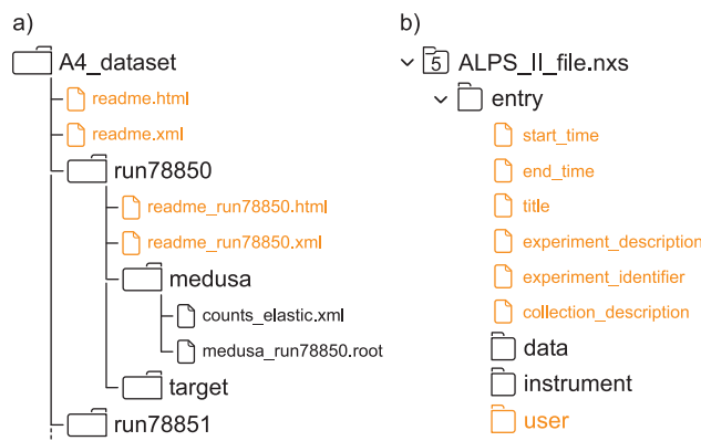
Figure 2: a) Schematic structure of the A4 raw data set after being improved for publication. The XML and HTML readme files at the top level and run level (orange) are added to provide context information and to span a network of links allowing human agents to browse the content. b) Proposed structure of the ALPS II NeXus-like HDF5 file with context related data fields and the user group, containing contacts to the experimental team, at the top-level (orange).
