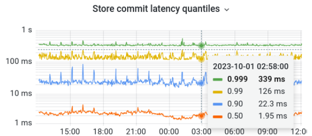
Figure 2: Quantiles of the duration between the receive of a Channel Access event update from the network and the commit confirmation for that update by the database server. Shown are 0.999, 0.99, 0.90 and 0.50 quantiles.
