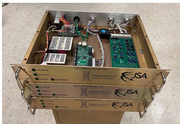
Figure 9: Commercially completed two channel helium flow meter chassis, 12 were fabricated
