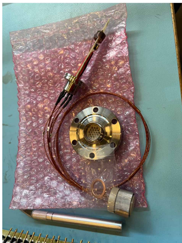
Figure 4: Final sensor configuration mounted on blade for installation into the return U-Tube.
