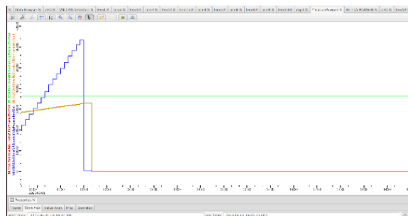
Figure 14: Using side-loaded test FEM firmware to remove known miscounts, no UpFrameErrCnt LVDS errors were observed during a 5 day test run at the beamline.
