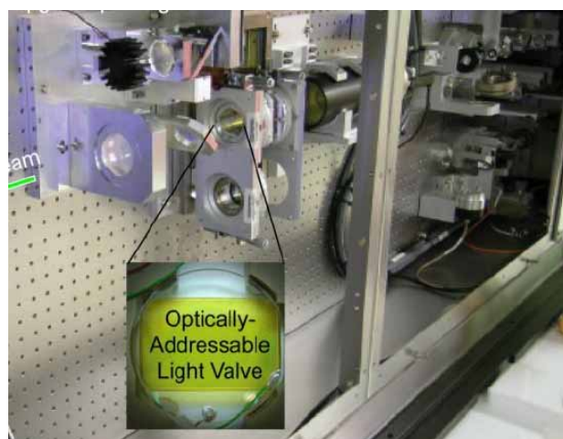
Figure 6: PSS in NIF Pre-amplifier Module (PAM).
