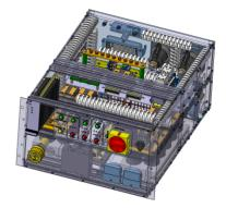
Figure 5: Capacitor Charger and Protection Unit.
