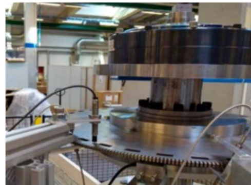
Figure 6: Wheel rotation speed sensor mounted to detect holes on the notch wheel around the target wheel shaft.
