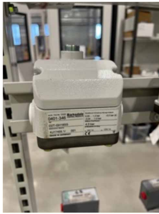
Figure 7: Monolith pressure switch.
