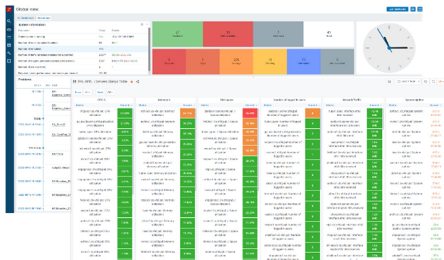
Figure 5: Control-related server monitoring system using Zabbix.
