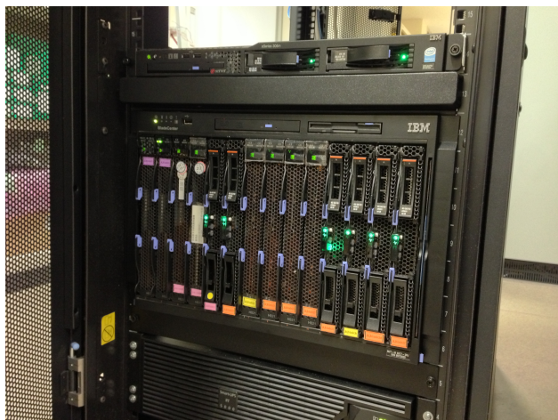
(a) An enclosure populated with 14 blades.
