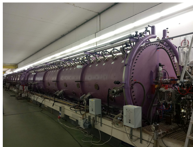
Figure 1: The Alvarez type main linear accelerator of the UNILAC went into operation in 1975.
