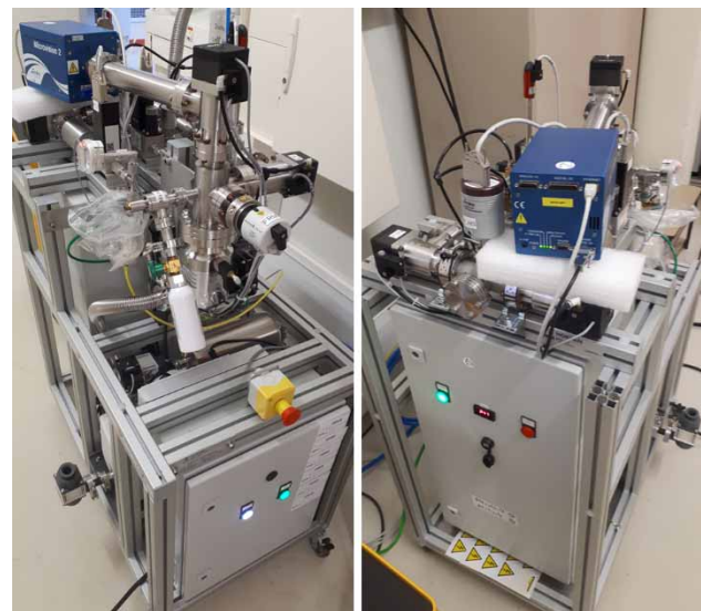
Figure 1: Mobile pumping units.
