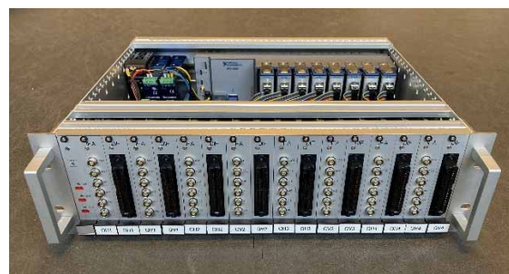
Figure 2: A photograph of a pilot subrack for the replacement of Bitbus based controllers using an NI-cRIO controller and custom-made DIF and IFA cards.
