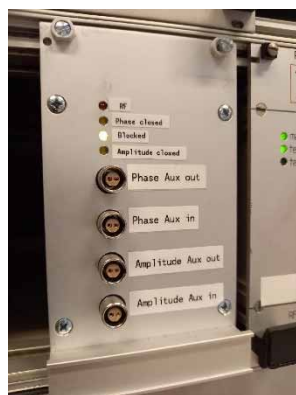
Figure 6: Photograph of a prototype of the new RF analog regulation system in which several modules are integrated into one.
