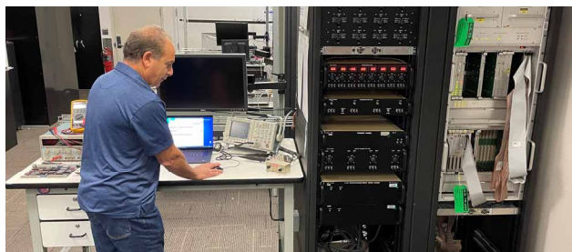
Figure 15: Motor driver and motion control board tests at an Alignment Control test station. Credit: LLNL.
