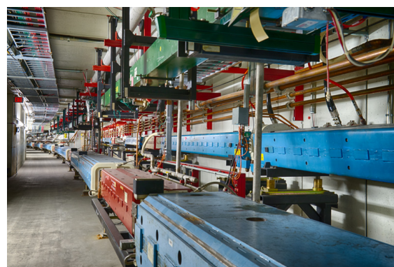
Figure 1: The Main Injector enclosure. Main Injector (bottom), Recycler Ring (top), P1 extraction beamline (middle).
