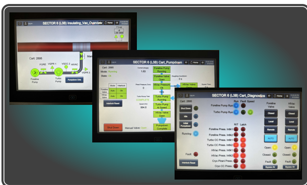
Figure 6: Example of PLC HMI screens.
