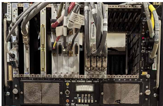
Figure 3: CAMAC Crate to be replaced by Moxa ioThinX.
