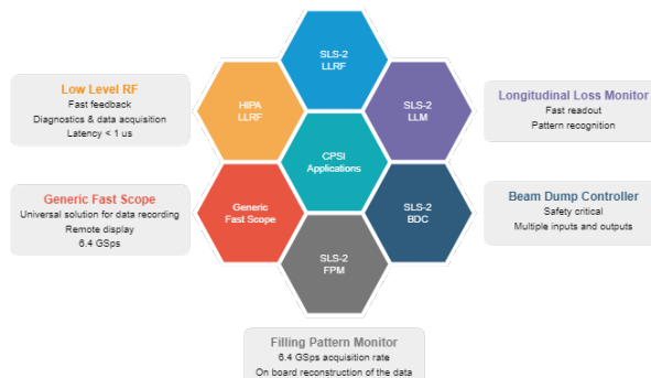
Figure 7: Diagram of accelerator applications that utilized CPSI-S.0 Hardware at PSI.
