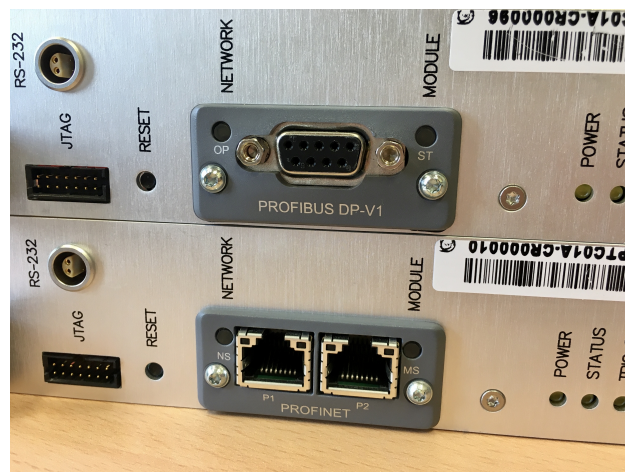
Figure 5: Two PTC cards with different network modules installed, e.g. PROFIBUS (top) and PROFINET (bottom).
