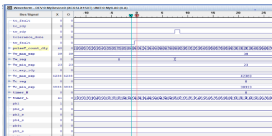
Figure 3: PW fault signal is asserted one clock (80.5 MHz) after presented pulse counter (pulseT_count_dly) is larger than expected maximum value of PW ( T_{w\_max\_exp} = 39 ) before PW count done signal is asserted ( tw\_rdy ).
