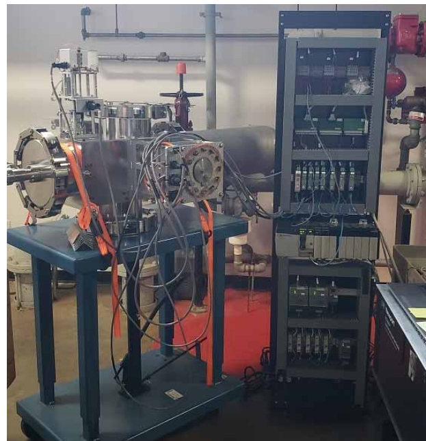
Figure 3: PLC test stand used on spare primary foil changer.
