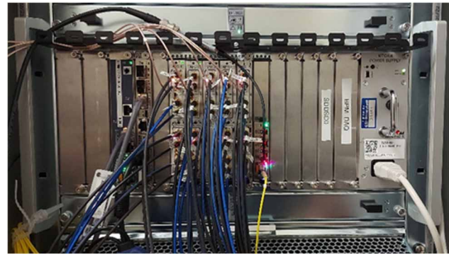
Figure 2: CRYRING@ESR Beam Position Monitoring system using AFC V4 FMC carrier modules with 250MSPS/4Ch/16 Bit ADC FMCs.
