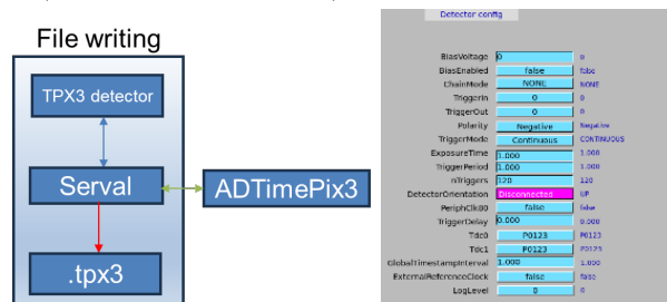
Figure 1: (left) ADTimePix3 configures SERVAL for writing .tpx3 raw files. (right) Detector parameter configuration control screen.
