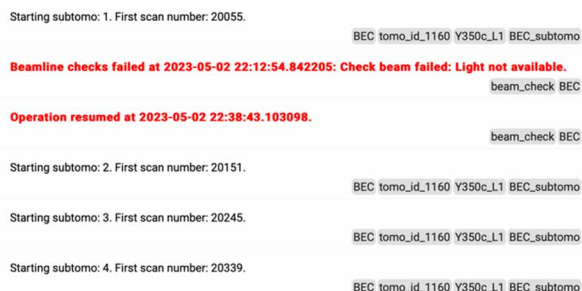
Figure 6: Logbook excerpt. Logbook entries can be further annotated using tags to improve the search results or filter the current logbook to only a subsection of entries. By integrating SciLog into BEC, beam checks can automatically report to SciLog and precisely track the time e.g., a beam loss occurred, simplifying the data analysis later on.
